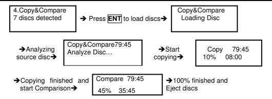
• The Compare Disc function serves as a bit-by-bit Comparison between Master Reading Source and the copied discs inside the writer trays. This operation ensures that all of the copies are completely identical to the Master Reading Source.
