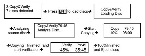
• The verification process makes a **Disc Readability Check**. This operation will check the master disc and the copied discs' readability to make sure all of the copies are readable.
